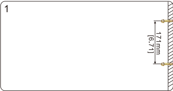
1. Drill 2x \varnothing 15 hole for expanded screws, and fix them to the wall. (Horizontal distance: 171mm)
